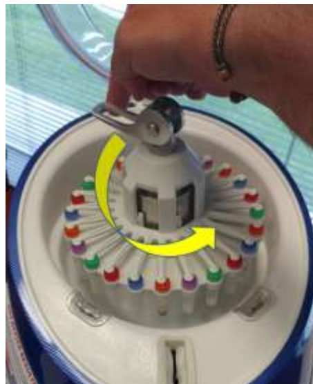
Figure IV-16 Unscrew Unlocked Cam Lock
