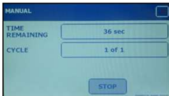
Figure V-11: FastPrep-24 5G Countdown Display during Manual Assay Run
