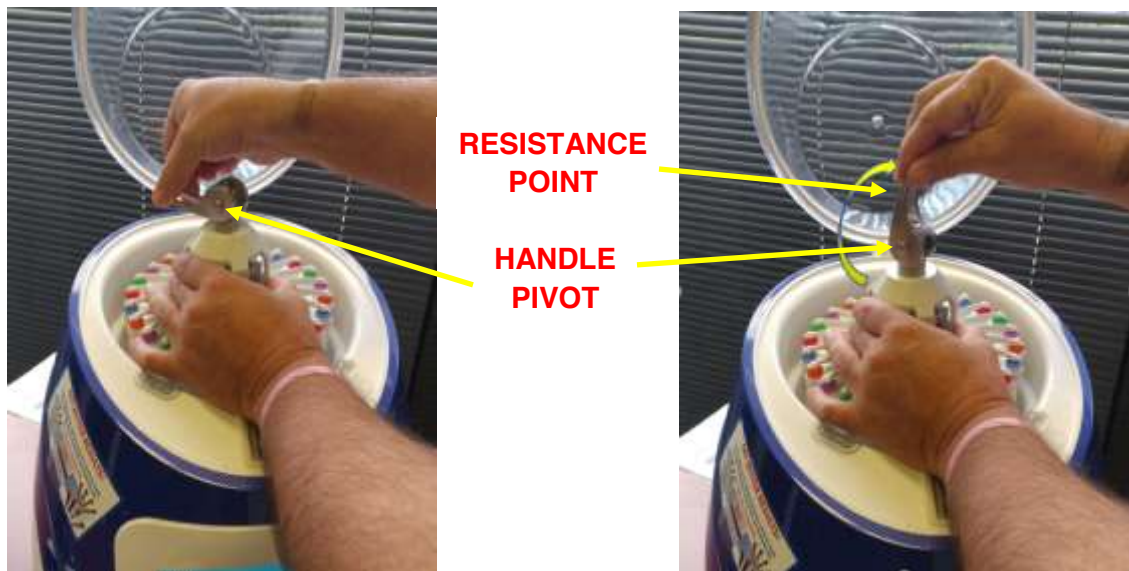
Figure IV-11: Lift Handle Around Pivot
