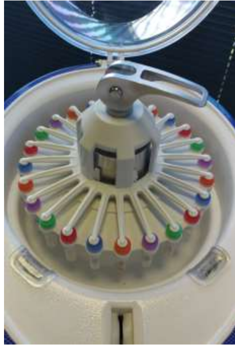
Figure IV-13: Cam Lock Fully Locked
