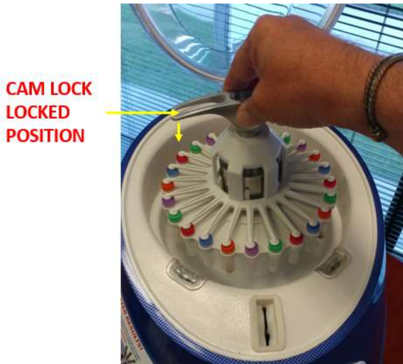
Figure IV-7: Thread Cam Lock on Ratchet Bolt
