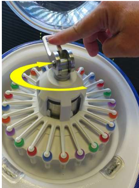
Figure IV-10: Rotate Unlocked Cam Lock 180 Degrees
