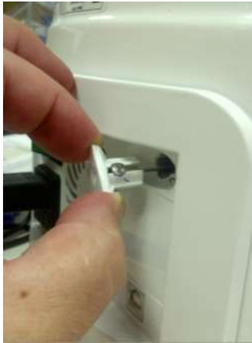
Figure III-2: 'Manual Dome Release Cable'
