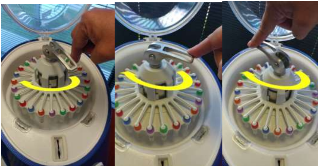
Figure IV-8: Rotate Cam Lock Clockwise
