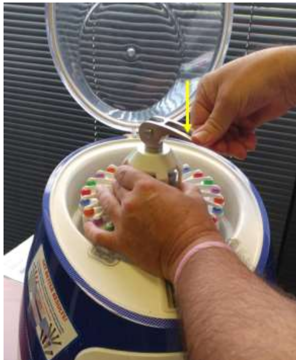
Figure IV-12: Press Handle Down Until Stop
