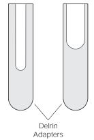
A Delrin adapter in a rotor cavity or bucket will significantly change the radial distances measured in the tube. The equations below can be used to determine  $r'_{\text{max}}$  and  $r'_{\text{min}}$  for a given rotor with a Delrin adapter. Table 2-3 lists adapter dimensions used in the equations.
