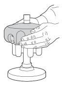
2. Carefully lift the rotor with both hands (do not carry a rotor with hook-on buckets by the rotor adapter; the buckets may be dislocated, resulting in an unbalanced rotor, spilled sample, and failed or collapsed tubes) and lower it straight down onto the drive hub. Make sure that the rotor pins are at a 90-degree angle to the drive hub pins. Careful installation will prevent disturbing the sample or tripping the imbalance detector.
