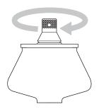
4. Place the lid on the rotor and tighten it, as firmly as possible, with the handle. Screw the handle down clockwise to fully compress the O-rings.
