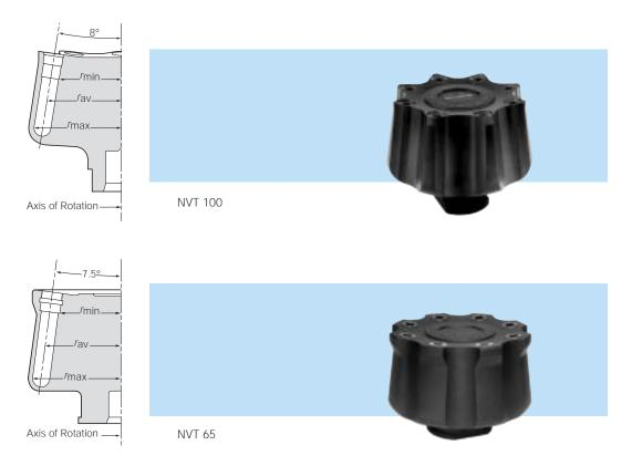
Figure 6-2. Near Vertical Tube Rotors
