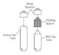
• If *Quick-Seal tubes* are being used, install spacers and/or floating spacers over sealed tubes (refer to the applicable rotor manual). The particular type of tube support for Quick-Seal tubes in fixed angle rotors depends on the length of the tube, but the top of the tube must be supported. Leave cavities without tubes completely empty.
