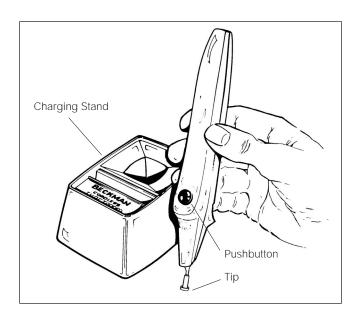
Figure 3-2. The Cordless Quick-Seal Tube Topper
