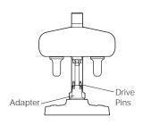
1. Note the location of the two small indentations on the rotor adapter (or the mechanical overspeed devices on older rotors). Their position indicates the location of the drive pins.
