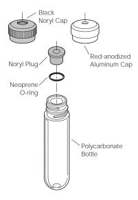
Cap bottles with three-piece cap assemblies as follows:
