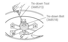
Rotor Tie-down Bolt (339031) Spanner Wrench (870666) • JS-4.2A and JS-4.2SMA—secure the rotor to the drive hub with the tie-down bolt (368518). Tighten the bolt with the tie-down tool (368521), then remove the tool.
