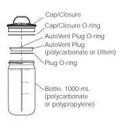
Bottles are available in polycarbonate (hard and clear), polypropylene (translucent), and polyallomer (translucent). Sealed polyallomer or polycarbonate bottles, available for most fixed angle rotors, have a three-piece liquid-tight cap assembly. Other bottles have screw-on caps. Cap assemblies should always be removed before autoclaving bottles. Bottle selection depends on the rotor in use and the specific application; refer to the applicable rotor manual.
