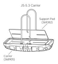
High-impact thermoplastic carriers are used in the JS-5.9 and JS-5.3 rotor buckets to provide support to labware during centrifugation and facilitate loading and unloading buckets. Each rotor bucket can carry a 96-well kit for high-throughput processing (such as a DNA or RNA kit), or standard microplates used in the serial dilution of small liquid volumes—up to five (JS-5.9) or six (JS-5.3) stacked 96-well polypropylene plates, two (stacked) deep-well plates, or one square-well plate per bucket.
