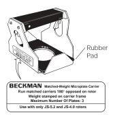
Carriers used with the JS-5.2 and JS-4.0 rotors are NOT interchangeable with those used with the JS-4.2, JS-4.2A, JS-4.2SM, JS-3.0, and JS-2.9 rotors. If you have more than one type of carrier, check the label on the side of the carrier to make sure that you are using the right one for your rotor. Table 5-2 lists carriers used with J6 rotors.
