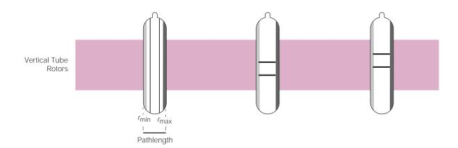
Figure 1-2. Particle Separation in Fixed Angle, Swinging Bucket, and Vertical Tube Rotors. Dark gray represents pelleted material, light gray is floating components, and bands are indicated by black lines.
