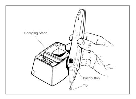
Figure 3-1. The Cordless Quick-Seal Tube Topper
