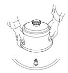
2. To remove the rotor, lift it straight up and off the drive spindle.
