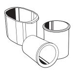
Polypropylene blood bag cups are available for use in swinging bucket rotors to obtain cell-free plasma for cell packing or for leukolyte depletion. Different sizes of cups are available to accommodate single, double, triple, or quad pack blood bags. Refer to the applicable rotor manual to determine the correct blood bag cup to use. Blood bag cups are autoclavable.
