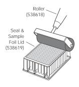
Seal & Sample aluminum foil lids (538619) have a bioinert adhesive backing, enabling complete plate sealing. The lids are presized for multiwell, deep-well, and square-well plates, and cause no reduction in well capacity. A 4-inch soft-rubber roller (538618) is required to ensure secure sealing of the foil lids.
