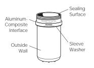
Cannisters used in some J-Lite rotors are made of lightweight carbon fiber epoxy composite. The lightweight cannisters make the overall rotor weight significantly lighter than a comparably sized all-aluminum rotor. Each cannister has a sleeve washer, made of Teflon¹ and Ultem,² which acts as a sleeve between the cannister and the aluminum rotor body. A lubricated ethylene propylene rubber O-ring inside the cannister closure helps create a secondary seal during centrifugation.
