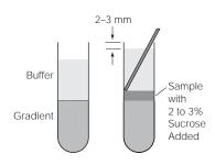
For *thinwall* tubes only partially filled with gradient, add a buffer solution to fill the tube to provide tube wall support. Although the gradient volume is reduced, sample volume is not changed.
