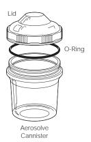
Aerosolve cannisters, used in the JS-4.3 swinging bucket rotor, are designed to minimize aerosol leakage and liquid spills. The cannister is transparent, enabling you to see broken labware and take proper precautions before opening the cannister.
