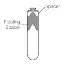
Quick-Seal tubes require spacers made of anodized aluminum, with or without floating spacers. The particular combination depends on the type of rotor being used and the tube size.
