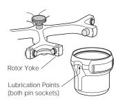
JS-4.2, JS-4.2A, JS-4.2SMA, JS-5.9, JS-5.3, JS-5.0, and JS-4.3 Rotors—Approximately once a week, and after cleaning and/or autoclaving, lubricate the pin sockets with a lubricant such as Paint On Graphite Lubricant (977212). Allow the lubricant to dry for at least 5 minutes before installing the rotor in a centrifuge.
