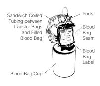
Different cups, color-coded for capacity identification, can accommodate single, double, triple, or quad pack blood bags. Refer to the applicable rotor manual to determine the correct blood bag cup to use. Do not pour liquid directly into blood bag cups. Fit blood bags into cups before loading the cups into the rotor buckets. Stuffing blood bags directly into the rotor while it is installed in the centrifuge can trip the imbalance detector.
