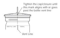
Place the plug on the bottle, then screw on the cap/closure by hand as tightly as possible. Tighten until the timing mark on the cap/closure is aligned with or goes past the vent line on the bottle.
