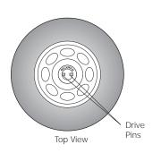
Currently produced J series rotors have drive pins in the drive hole. These pins mesh with teeth on the centrifuge drive spindle hub when the rotor is installed to ensure that the rotor does not slip on the hub during initial acceleration. Most drive pins are oriented horizontally (or angled) in the drive hole; however, some are oriented vertically.
