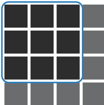
When performing image capture on the Amersham ImageQuant 800, it is possible to adjust the binning settings for either greater sensitivity or greater resolution. Increasing the sensitivity results in a decrease in the exposure time. The option for this is found under **Advanced settings** in the method window for all **Chemiluminescence** and **Fluorescence** imaging. To change the binning settings, use the following procedure.
