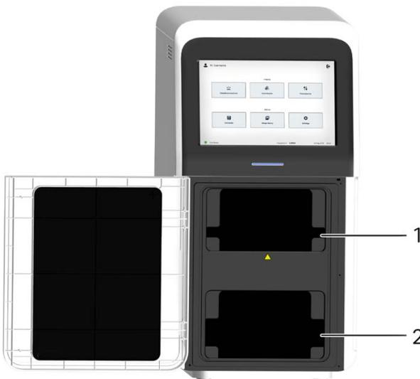
The position of the tray is detected automatically by the Amersham ImageQuant 800 control software and displayed at the bottom of the screen. The display is automatically updated if the tray position is changed.
