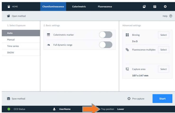
The **Tray position** indicator will display as **Upper**, **Lower**, **NP lens for plates**, and **None**.
